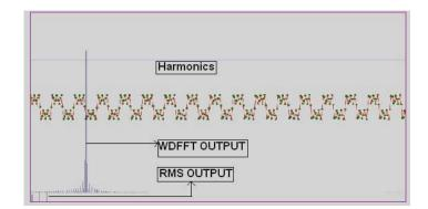
c) e(t) = A1\* Sin(wt) – A3 \*U1\*(t-T1)\*U2\* (t-T2)\*Sin(3wt)+A5\*Sin(5wt)+A7\*Sin(7wt) (Harmonics)
