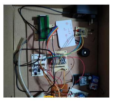
Fig 2. Prototype of proposed model
