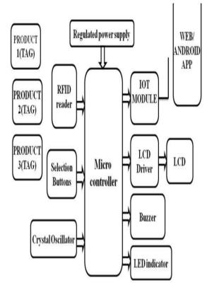
Fig 1. Block Diagram of the proposed model
