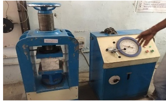
Fig. 4.1. Testing the cubes in compression testing machine.
