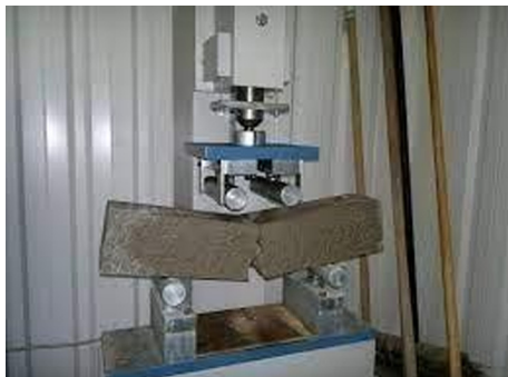
Fig. 4.3. Testing of beams.
