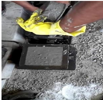
Fig. 3. Casting of Conventional Cube.
