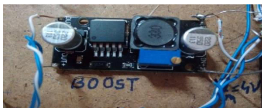
Figure-17. Hardware model of boost converter.
