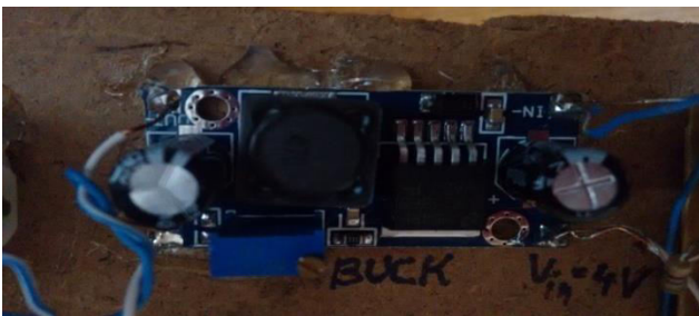
Figure-19. Hardware model of buck converter.
