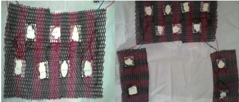
Figure 7. Peltier Plate Panels Connected.
