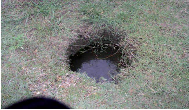
Fig 6.15 Rat Hole Mining for Placer Concentrations
