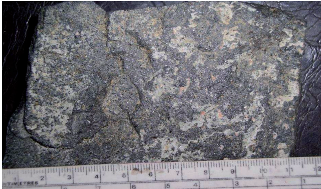
6.13 Granules of Corundum in coarse grained felsic rocks.
