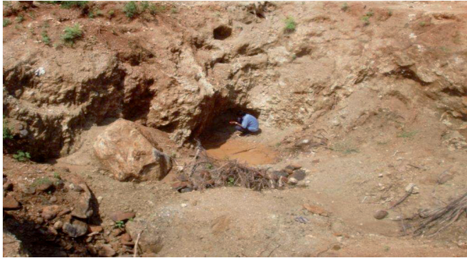
Fig 6.3 Insitu working Pit for Corundum
