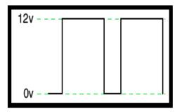
Solar array current is controlled by PWM so that it changes according to the battery's condition and the rate at which it recharges. As an example, imagine a voltage waveform like this: every second, it cycles between zero and 12 volts and back again.
