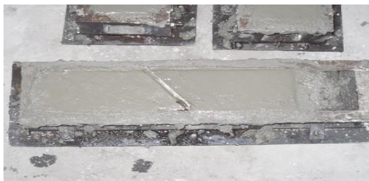
Figure 3. Process of casting prism making regular 45 0 angle by keeping a steel plate
