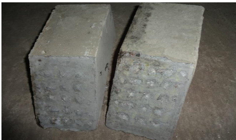
Figure 26. Failure of the specimen with rough interface reinforcement under slant shear test
