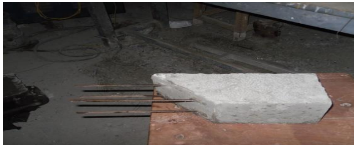
Figure 6. Specimen that had casted with 6mm diameter bars at 45 0
