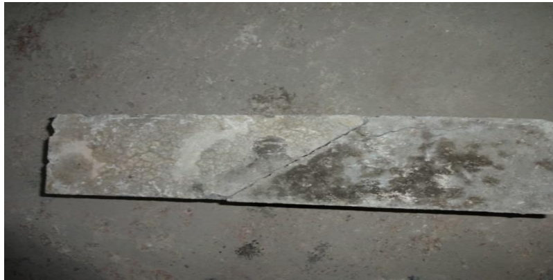
Figure 27. Failure of the specimen with under slant shear test
