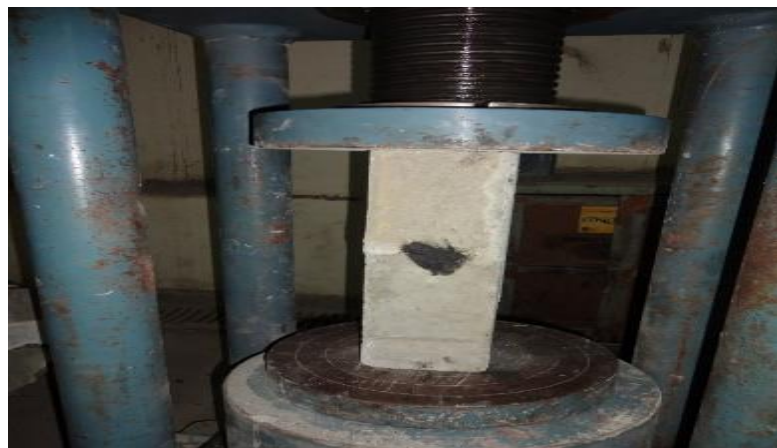
Figure 10. CTM prisms are tested under compressive strength
