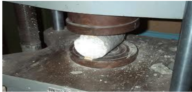
Figure 2. Split tensile test
