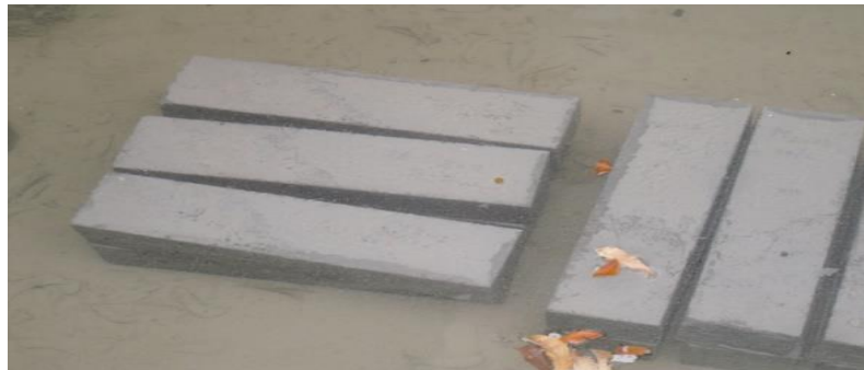
Figure 9. Specimen after adding new substrate to the old substrate kept for curing
