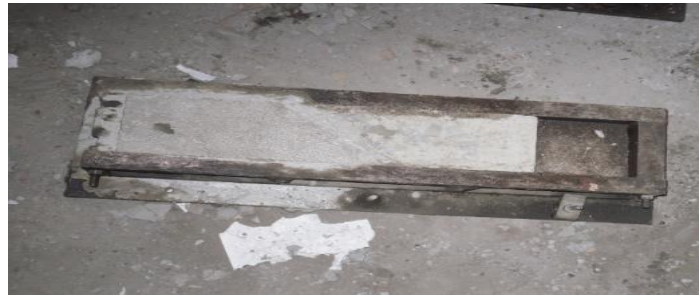
Figure 5. Casting of new substrates over the old substrate
