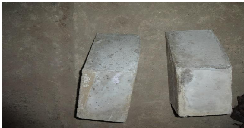
Figure 25. Failure of the specimen having smooth interface under slant shear test
