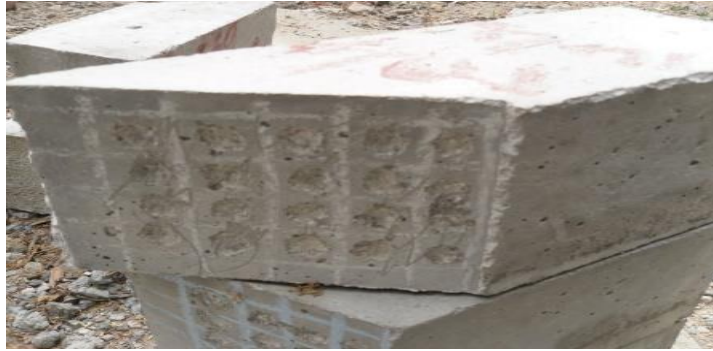
Figure 4. Specimen that had chipped at intervals after 28 days of curing at 45 0
