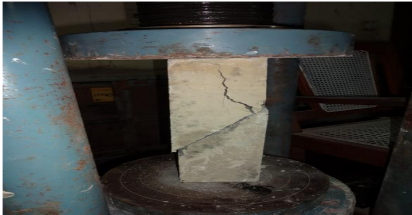
Figure 24. Failure of the specimen under slant shear test
