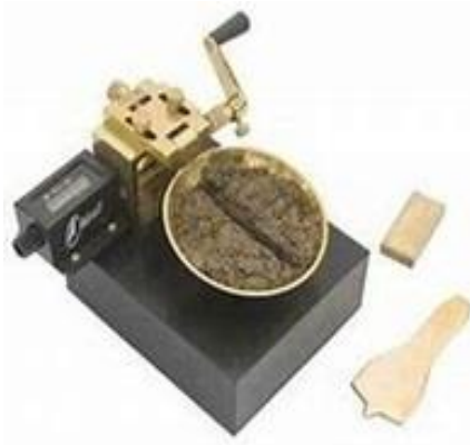
Figure 3. Liquid limit apparatus.
