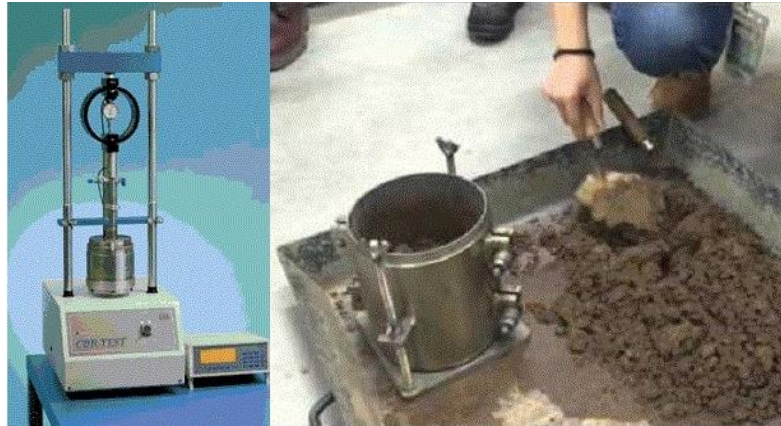
Figure 7. California bearing ratio (CBR) test.
