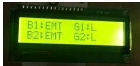
Fig. 4: LCD displaying the status of bins
