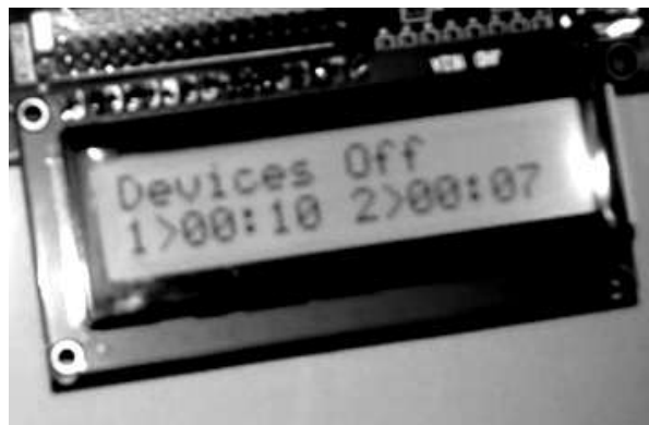
Fig. 8: LCD Output When Devices are OFF.
