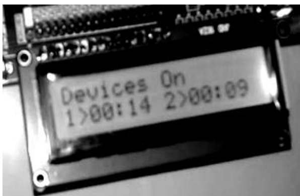
Fig. 7: LCD Output When Devices are ON.
