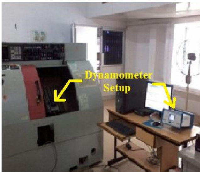
Fig. 1 CNC Machine with dynamometer setup.
